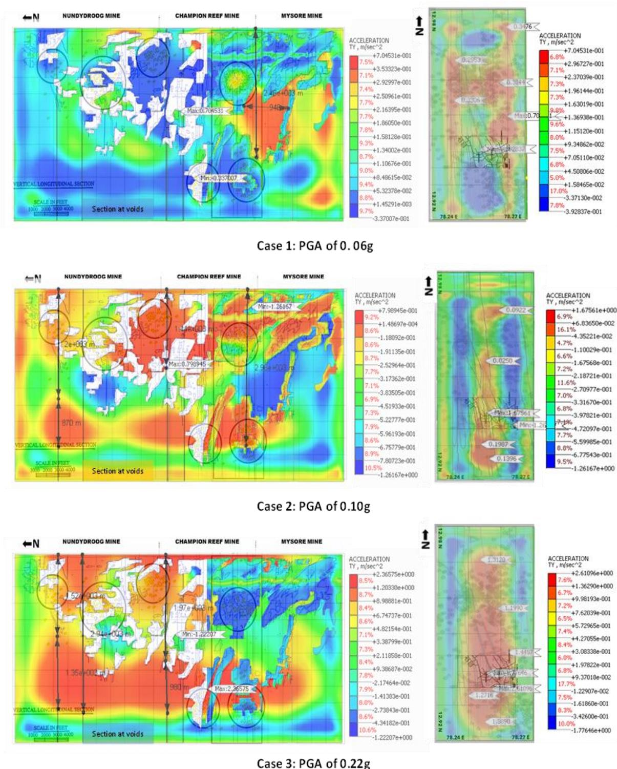
**Fig. 9: Zones of failure at void section and at surface w.r.t. field observations for all three cases**
