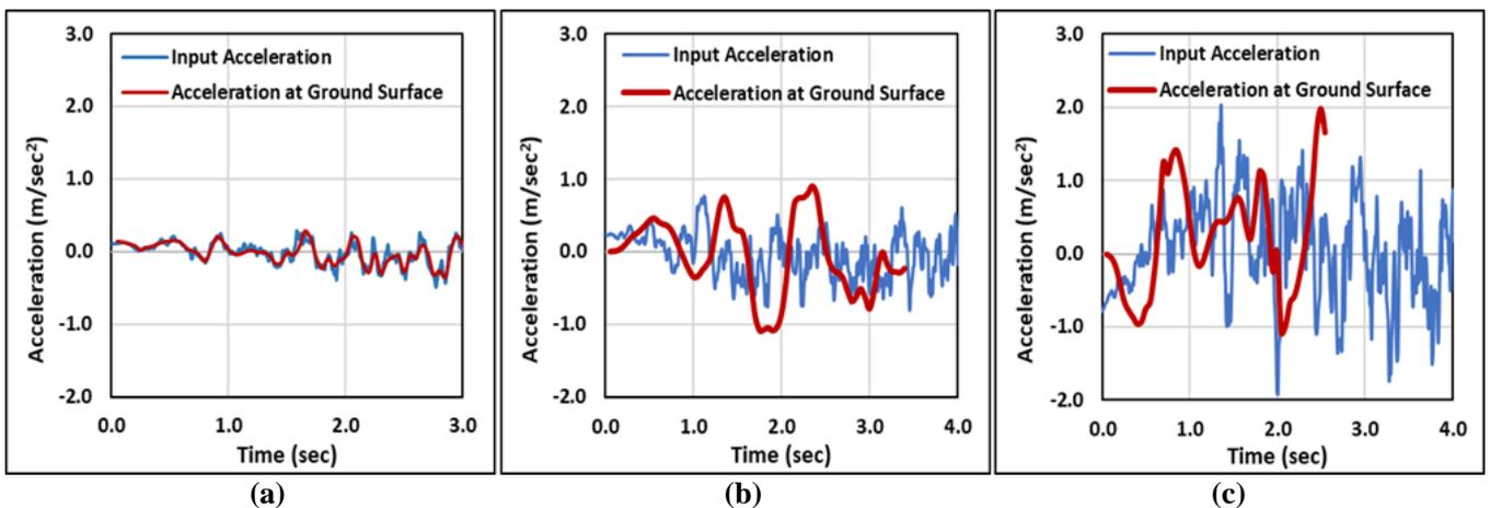
Fig. 7: Acceleration time histories at ground surface (a) Case 1 (b) Case 2 (c) Case 3
