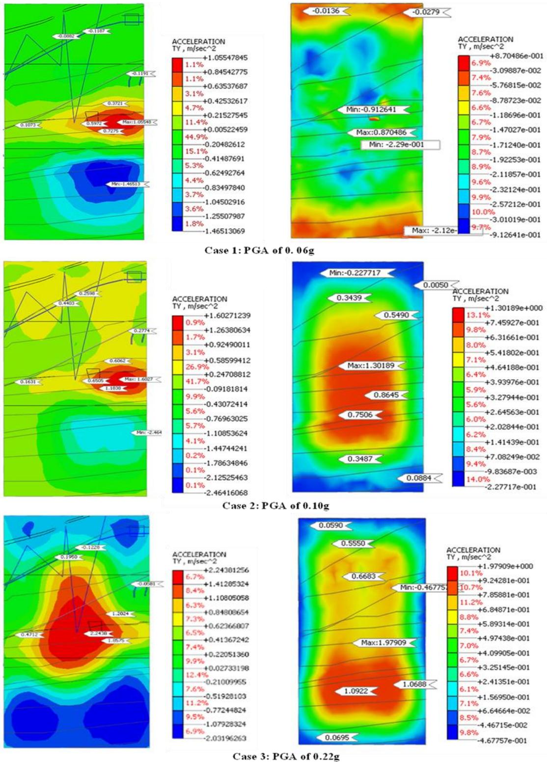
Fig. 11: Vulnerable zones at surface for section with fault (left) and section without fault (right)
