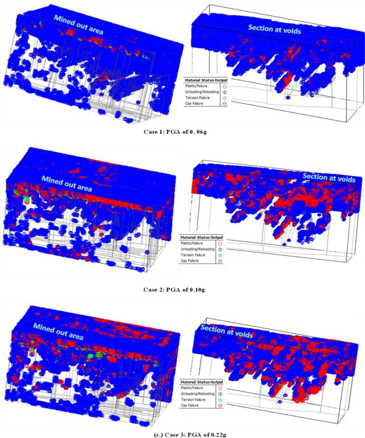
**Fig. 5: Plastic and Tensile failure zones for all three cases of PGA**
