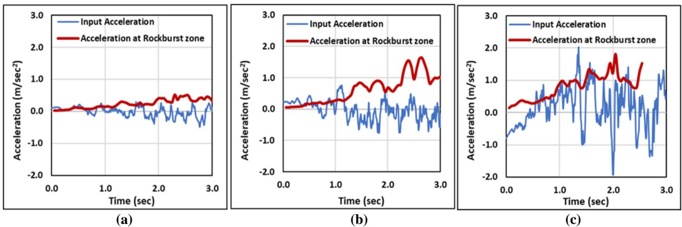
Fig. 6: Acceleration time histories at rock burst zone (a) Case 1 (b) Case 2 (c) Case 3
