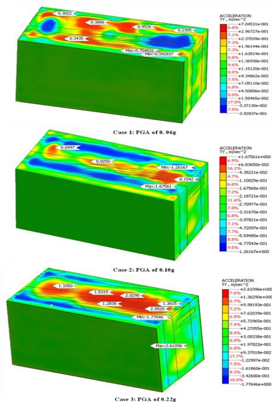
**Fig. 8: Accelerations observed at the ground surface for all three cases**
